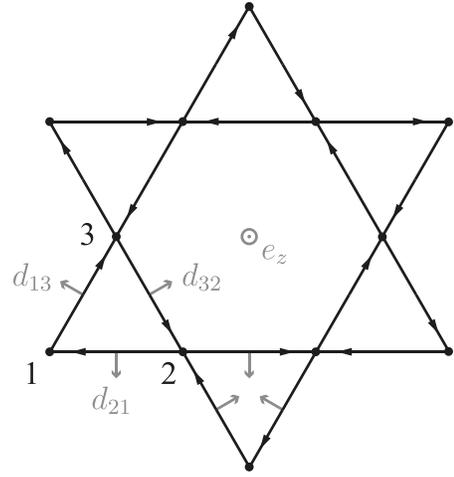
FIG. 2. **DM interactions on the kagome lattice.** On each lattice bond, the orientation of the DM coupling  $(De_z + D'd_{ij}) \cdot (\mathbf{S}_i \times \mathbf{S}_j)$  is defined by the black arrows pointing from site  $i$  to  $j$ . The orientation of the in-plane component of the DM vectors is different for up-pointing and down-pointing triangles, as indicated by the gray arrows. The vectors  $e_z$  and  $d_{ij}$  have unit length.
